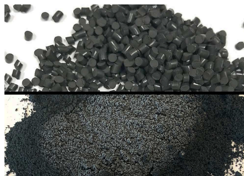
Fast milling of black Fluoro-carbon rubber (FKM) by embrittling the sample in two 125 ml jars at -100 °C.
